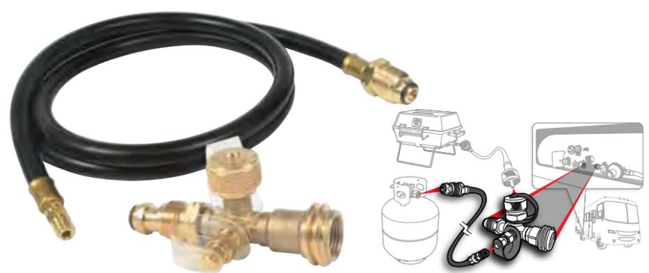
**90° PROPANE TEE WITH 12' HOSE** Connects to camper or trailer propane cylinder to allow connection of an additional propane appliance such as a tabletop grill, camp stove or lantern. Provides thermal protection in case of fire and excess flow protection in case of broken gas line. Includes propane tee (Type 1 Acme nut x female P.O.L. and male acme thread x 1"-20 male throwaway cylinder thread) and 12' extension hose with male x female swivel 1"-20 female throwaway cylinder threads.
