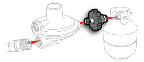
**QUICK-CONNECT FULL-FLOW PLUG** For use in low-pressure propane systems to add a convenient connect/disconnect method. 1/4" Male NPT x Male Quick-Connect.
