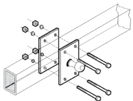
**SWAY CONTROL PARTS** Replacement parts for Eaz-Lift 48380 and 48381.
