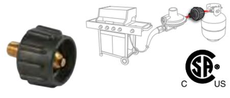
**P.O.L. PLUG ADAPTER** For use on a 20 or 30 lb refillable tank to connect cylinder to regulator. Converts 1/4" NPT to female P.O.L. Provides excess flow protection in case of broken gas line. Soft Nose P.O.L. x 1/4" Male NPT.
