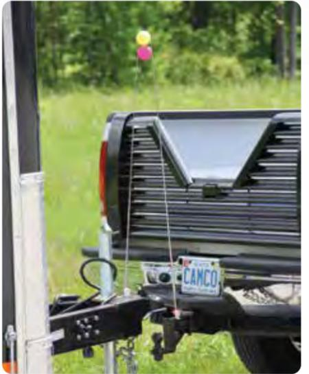
**BALL MOUNTS** Ball mounts are 2" x 2" and function as a weight carrying hitch. Ball mounts create a ball platform for attaching a hitch ball. The ball mounts or utility hitch bar length are determined by measuring from the center of the pull pin to the center of the hitch ball hole. The drop or rise is determined by measuring from the top of the mount to the top of the tongue. All 2" x 2" ball mount shank holes are 1", except 48282, which has a 3/4" hole.
