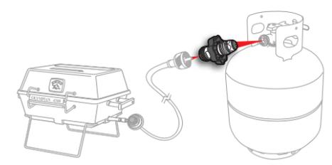
**PROPANE Y ADAPTER WITH HANDWHEEL** For use on a 20 or 30 lb refillable propane tank. Allows you to operate two appliances such as a Campfire and a grill at once from the same cylinder. Provides excess flow protection in case of broken gas line. Male Soft-Nose P.O.L. x Two 1"-20 Male Throwaway Cylinder Thread Connections.
