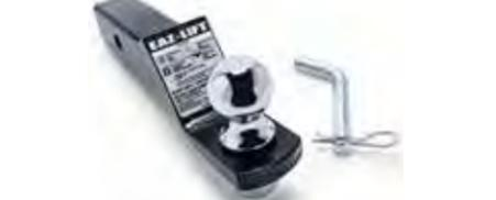
**COMBO BAR** 2" x 2" x 1/4" wall with collared tube, used to create under-car receivers for vehicles where standard or frame hitches are not available. Can be bolted or welded to vehicles undercarriage. Sized and punched to fit all common weight distributing hitch ball mounts or utility ball mounts. \*Wt. carrying only with 24" to 48" combo bar when properly installed. Fits 2" x 2" receiver.
