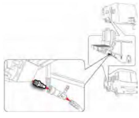
**GAS GAUGE/LEAK DETECTOR** See at a glance when your propane pressure level is low. Type 1 for gas grills, RVs and boats. Fits all propane tanks manufactured after 1995. Provides thermal protection in case of fire and excess flow protection in case of broken gas line. Acme Nut x Acme Thread and Female P.O.L.
