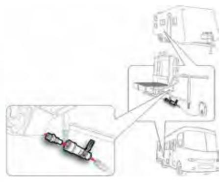
**GREEN PROPANE ACME NUT** 200,000 BTU/hour. For use on a 20 or 30 lb refillable propane tank to connect to a regulator/hose assembly. Provides thermal protection in case of fire and excess flow protection in case of broken gas line. Acme nut x 1/4" NPT.
