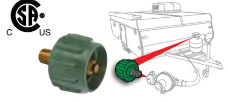
**BLACK PROPANE GRILL ACME NUT** 70,000 BTU/hour. For use on a 20 or 30 lb refillable propane tank to connect to a regulator/hose assembly. Provides thermal protection in case of fire and excess flow protection in case of broken gas line. Acme nut x 1/4" NPT.
