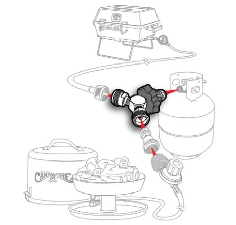
**PROPANE QUICK-CONNECT KIT** For use in low-pressure propane systems to add a convenient connect/disconnect method or to add an additional safety shut-off. Valve: 1/4" Female NPT x Female Quick Connect; Full Flow Plug: 1/4" Male NPT x Male Quick-Connect.
