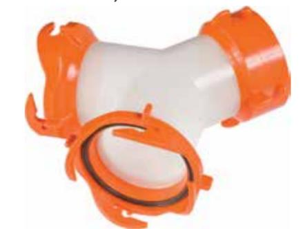
**RHINOFLEX RV SEWER HOSE SWIVEL BAYONET FITTING** Designed with four sturdy prongs that lock into position. Easy-grip wings for quick connect and disconnect. Built-in gasket for an odortight connection without hose clamps. Stores in 4" square bumper. Complete with reusable locking ring. Patented. RhinoFLEX hose not included.
